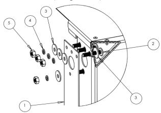
Attach the vent hood directly into the spacer through the mounting holes located on the rear hood cover plate. Fasten and tighten all hex nuts. Reference the parts list below to identify the hardware included with your wall mount spacer.
