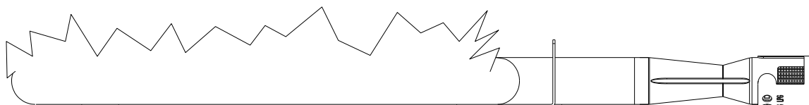
Poor Combustion: wavy, yellow flames-too little air
